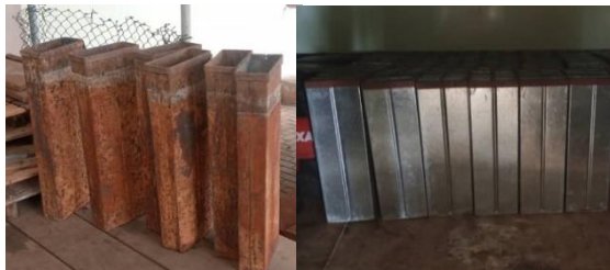
Old ice-making can that leaks water (left) and new ice-making can that was purchased (right)
