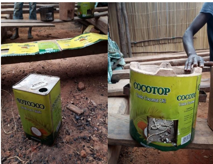
Improved kitchen stove made with recycled materials.
