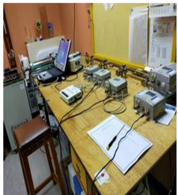
Digital barometer calibration namely (PTB series) JICA provided Tough Book HP laptop and calibration equipment.
