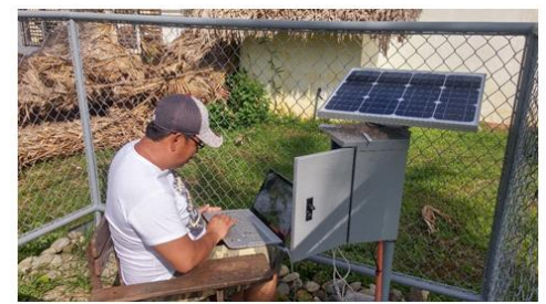
An Automatic Rain Gauge equipment installed for radar calibration and quantitative precipitation estimation
