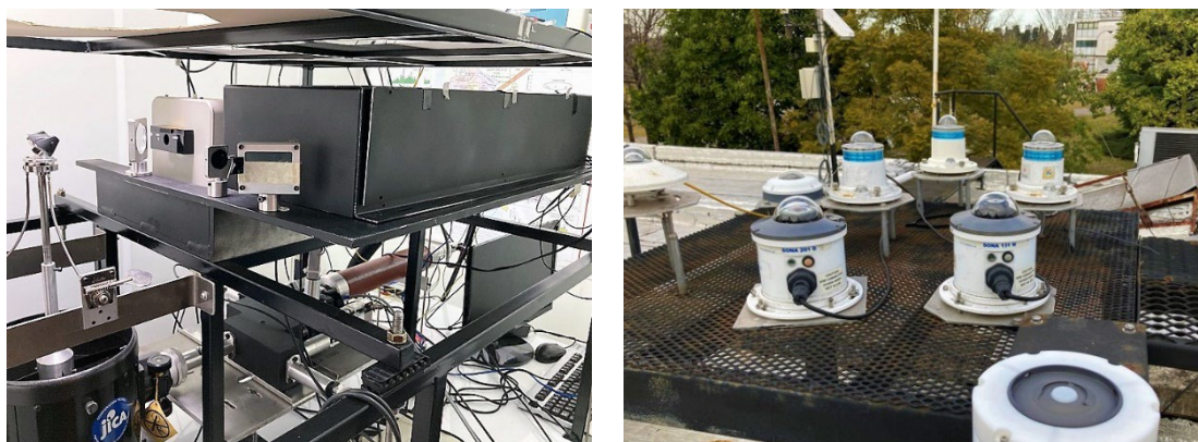
SMN's LIDAR instruments (left), instruments for UV etc. (right)
