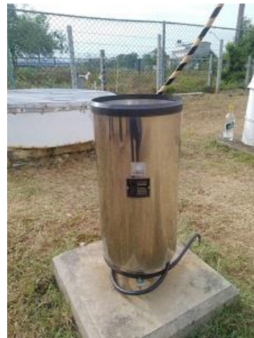
Rain gauge of Polonnaruwa Station
