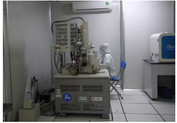
Scanning electron microscope and energy dispersive x-ray spectroscopy installed at INT, Ho Chi Minh City
