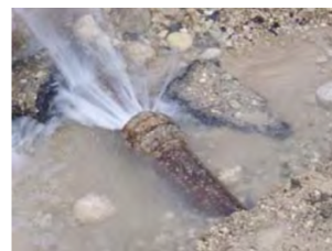
Photo 2: Leakage due to broken pipe joint
