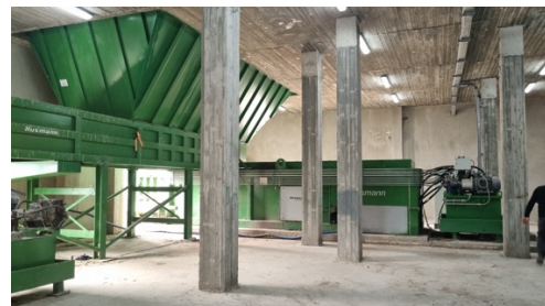
Indoor Hopper and Compressor at Al Taybeh TS
