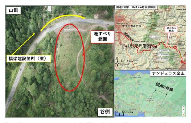
Note: The bridge construction site is planned to be shifted to the mountain side,
