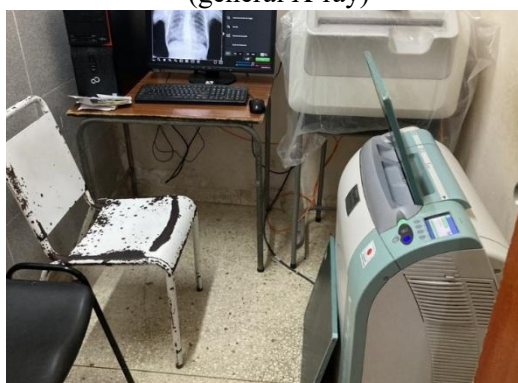
Photo 3. CR reader reading images from cassette
