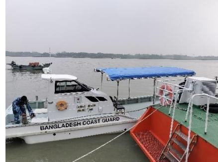
Photo3: 10m type rescue boats equipped with a canopy (Source: the external evaluator)
