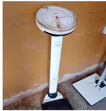
Photo 7: A Broken Weighing Scale Placed in the OPD of Gulu RRH (source: taken by the evaluator)
