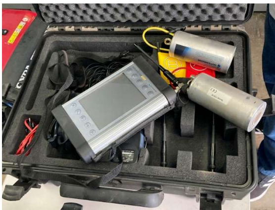
Photo 5. Leak detection equipment
