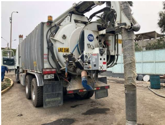
Photo 3. A hydro-jet truck
