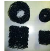
Anaerobic filter media
