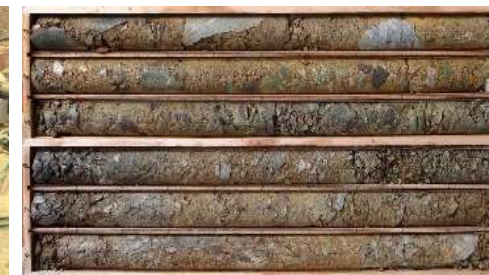
Core samples of landslide layer
