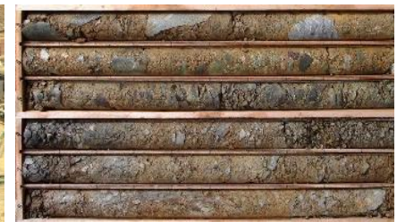
Core samples of landslide layer
