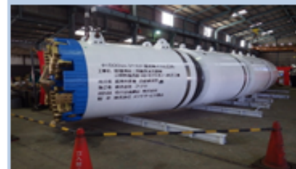
ESS Tunnel Boring Machine
