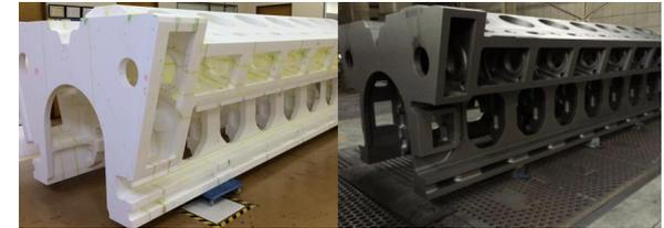
Mass produced products made with the FMC process
