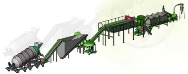
Production line of recycled PET pellets
