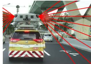
Acquiring 3D point cloud data* *integrated with XYZ coordinates.
