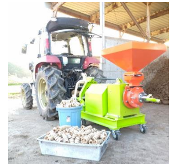
Tractor-driven rice husk briquette machine
