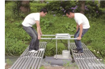
Power generator "Cappa" Can be carried by 2 adults, and immediately start power generation
