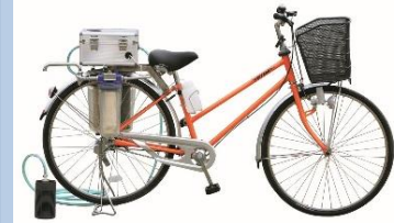
“Cycloclean”, Water Purification System loaded on a Bicycle
