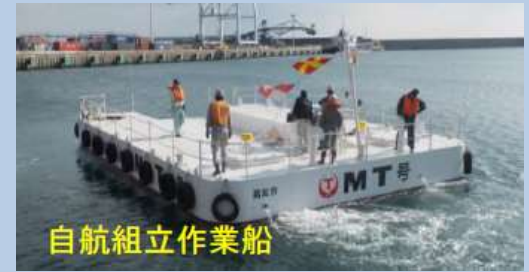
Sectional self-propulsion work barge
